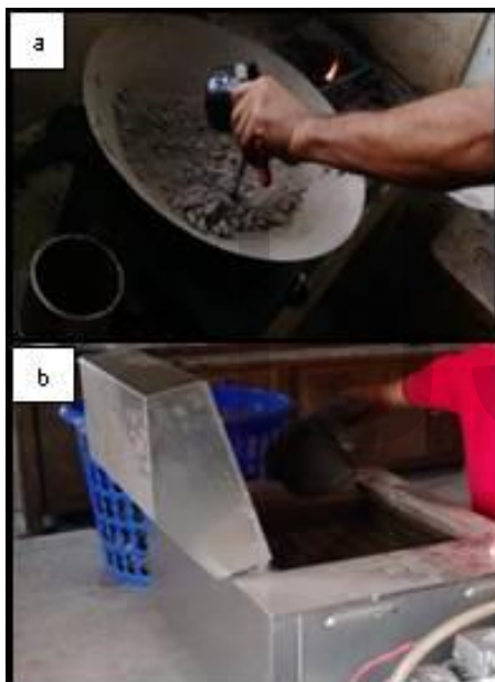
Fig. 3: Photo view of (a) materials mixing (b) sample placing in water
